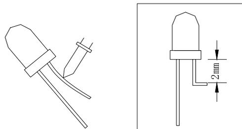
2) Forming lead should be carried out prior to soldering and never during or after soldering.
